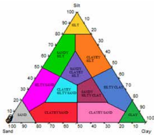
Fig. 2. Trilinear plots of sand, silt and clay ratio, of Kovalam beach sediment samples (after Trefethen, 1950)
